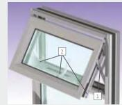
A turn of the handle operates the shootbolt locking mechanism and drives high strength brass alloy bolts into the window frame into die-cast keeps in the outer frame. The locking mechanism also offers a lockable 'night-vent' position.
